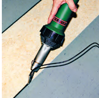
The TRIAC S hand welding tool, used for welding linoleum, equipped with a speed weld nozzle.
