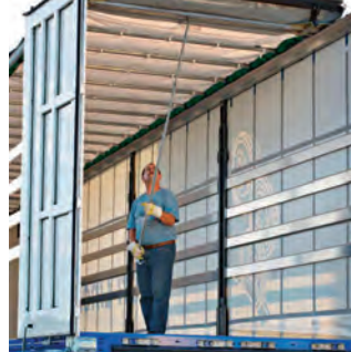
Tarpaulin bows for fixed and sliding rooftops of lorries (Pictures: Krone).
